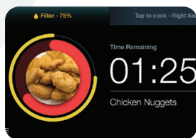
Red ring indicates cook time progress; gold ring indicates remaining oil life to filter
