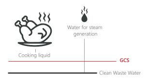
99.9% of the liquids from cooked products are collected by the grease collection system and do not get into the waste water.
