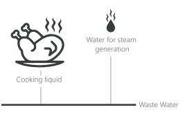
Liquids from cooked products mix with other liquids in the cooking chamber and get into the waste water.
