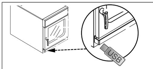
The USB interface is behind the cover on the bottom left of the housing.
