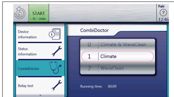
**Selecting a program** → Select a program by adjusting the roller.
