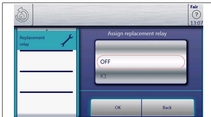
**Assigning the backup relay** → Select the defective relay by means of the roller.
