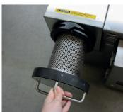
The next morning - step 1 Unlock the cap of the strainer and remove it by simply sliding it out. After cleaning the strainer, place it back in the tank.
