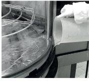
Weekly cleaning - step 3 Flush all three drip channels with hot water and degreaser.
