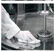
Weekly cleaning - step 4 To remove any lime scale deposits from the interior, use lime scale deposit cleaner or distilled white vinegar.
