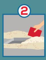
Remove the lug plug and push the used breading into the unit.
