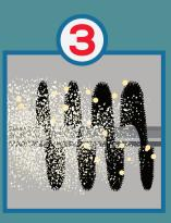
The brush forms an auger, sifting and blending breading while ejecting unwanted dough balls.
